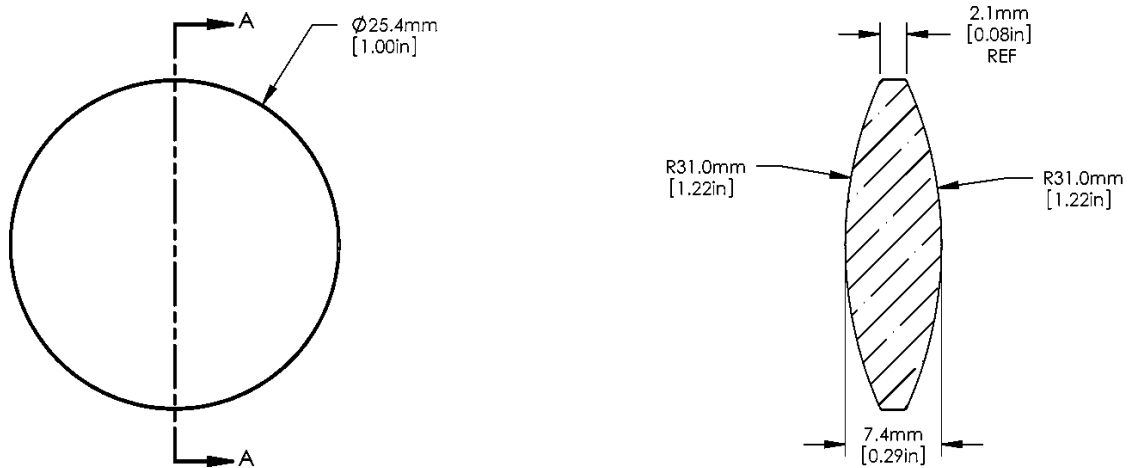
Figure K-14 Schematic of bi-convex lens (Part number: LB4879)
