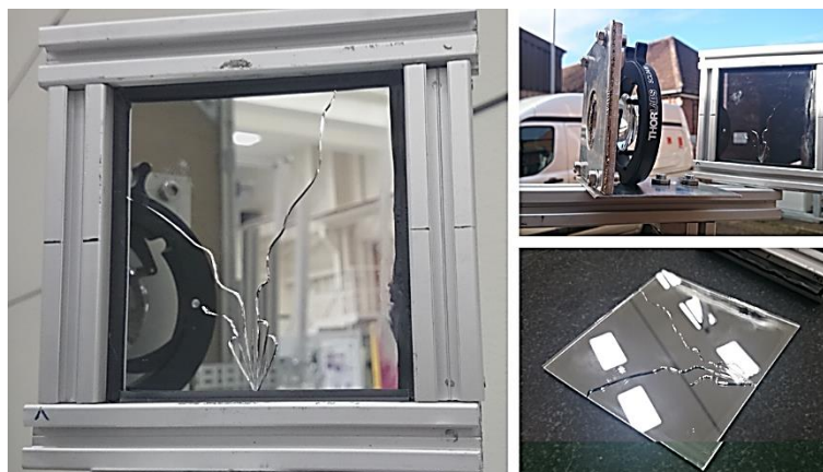
Figure 6-72 Cracks in the float glass-based 45° mirror
