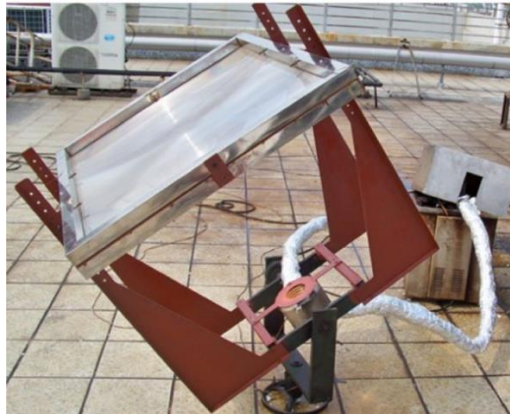
Figure 2-22 Xie's group point-focus Fresnel lens solar concentrator test rig (Xie, Dai and Wang, 2012)
