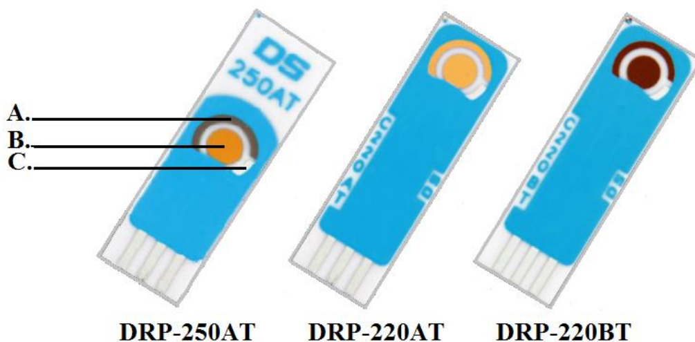
Figure 2.2: Screen printed electrode used in this project and their configuration of their electrodes. A. counter electrode; B. working electrode; C. reference electrode.
