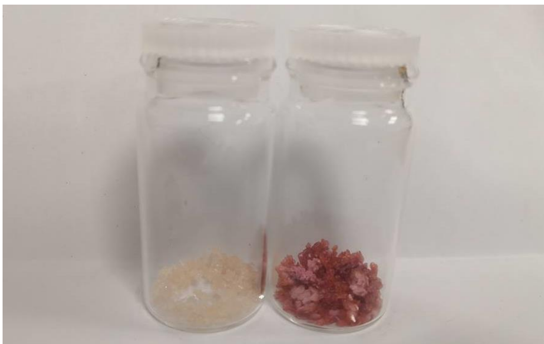
Figure 4-8 Dried cobalt alginate beads taken from the fifteenth run of B16 (left) and the first and second run of B16 (right), in which the different uptakes of cobalt can be observed from the change of colour.
