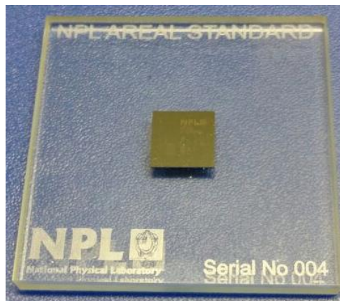
Figure 42. Calibrated step height artefact
