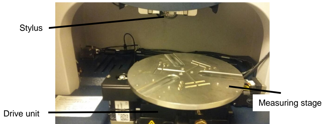
Figure 47. DektakXT close view
