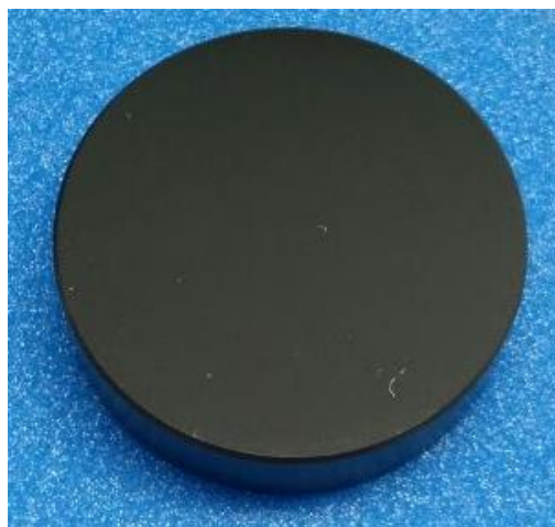
Figure 43. Calibrated optical flat standard
