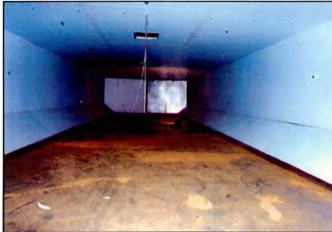
Figure 6.4-1: Test chamber furnished with original cargo lining material Cargo compartment based on an AIRBUS A340-200 forward compartment.
