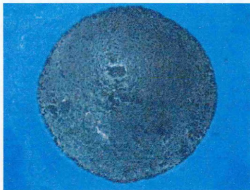
Figure 4.17 Photomicrograph of a sensor produced using the synQUAD™ dispensing platform
