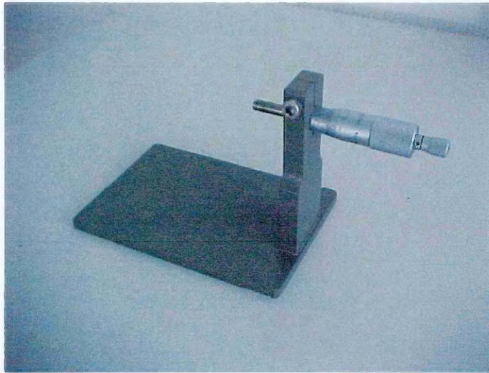
Figure 5.12 Micrometer fixed in purpose designed stand.
