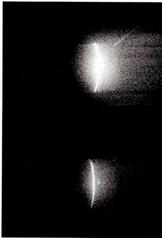
Figure 8.23: Unprocessed stripe compared to stripe processed through 'Laser Stripe 1a.vi'.
