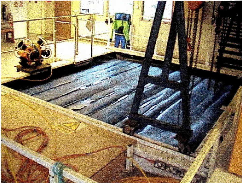
Figure 7.1: Cranfield test tank facility with cover over to remove ambient light
