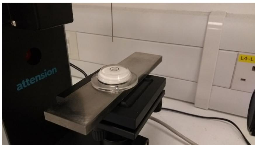
Figure 4.4.B. Working surface being balanced using a spirit level to ensure the surface is horizontal when a water droplet is applied.
