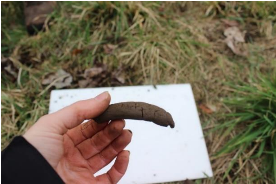
Figure 2.4 - Example of random soil sample (above) and ribbon (below) taken during preliminary soil texture test at the Silsoe field site following the methodology recommended by FAO (2000).
