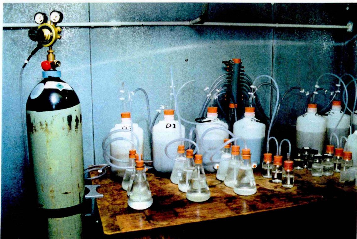
Figure 4.5 Experimental Apparatus Assembly for Biodegradation Study Incorporating the Titration Method of Carbon Dioxide Collection
