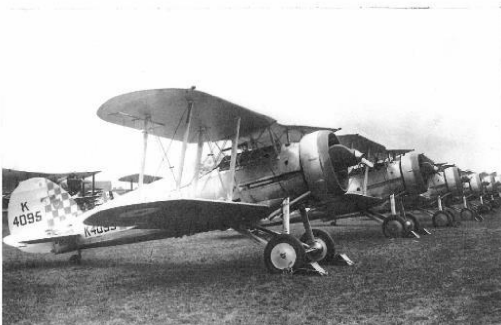
Above: Gloster Gauntlets of No 10 Squadron, also at Middeham in July 1935. The Gauntlet was introduced in May of that year, and with a top speed of 230mph was appreciably faster than its predecessor, the Bristol Bulldog. However, its open cockpit, bulky air-cooled radial engine and armament of only two fuselage-mounted machine guns all date back to World War 1. HU 26040
