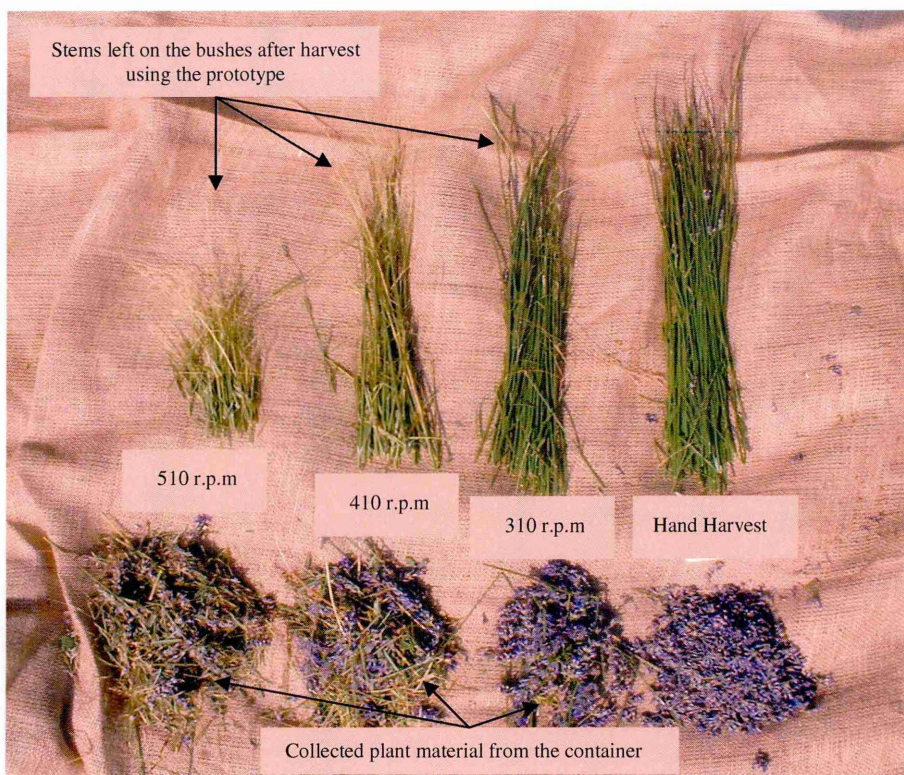
Plate 8.1: Effect of rotor speed on the amount of stem harvest 17
