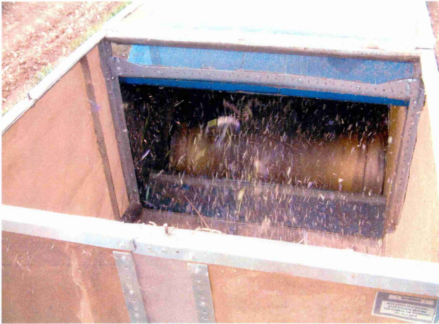
Plate 7.3: Crop flow through the hood exit
