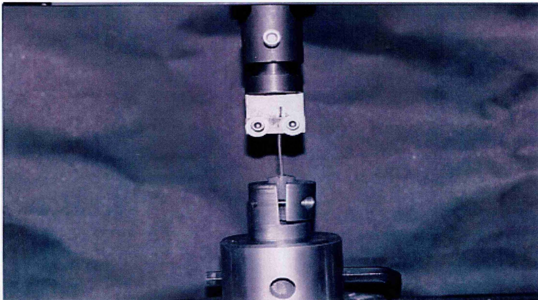
Plate 4.3: Experimental lay out for stem UTS test
