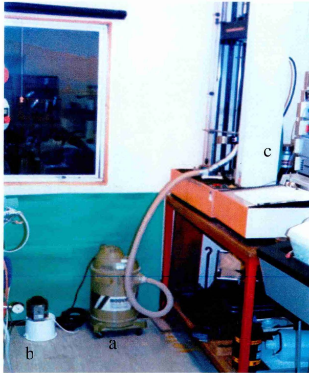
Plate 4.4: The equipment used for the airflow test (a= vacuum pump, b= variac 0-240 Volt, c= load cell)
