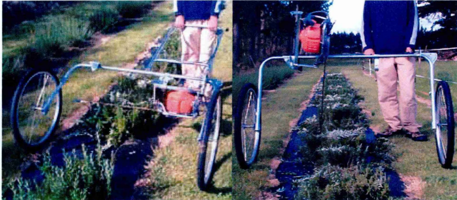
Plate 3.7: Portable hand held herb harvester
