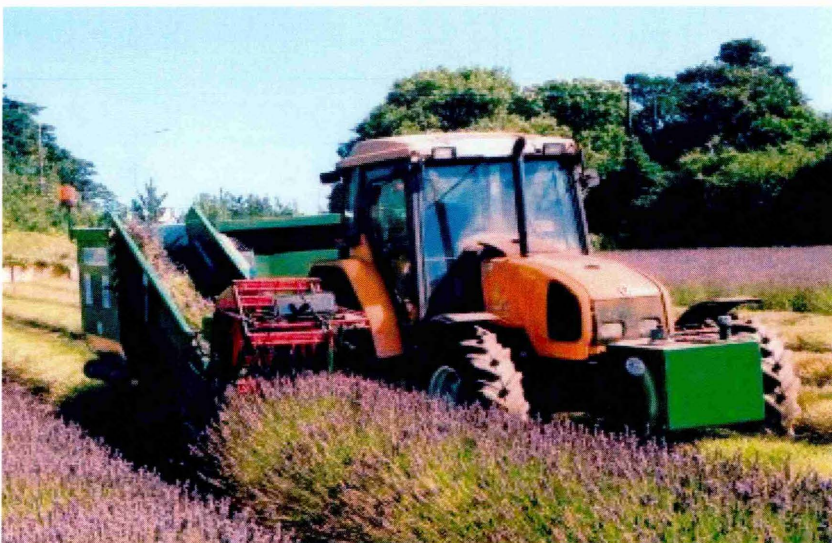
Plate 3.3: New type lavender harvester (Norflok Lavender)
