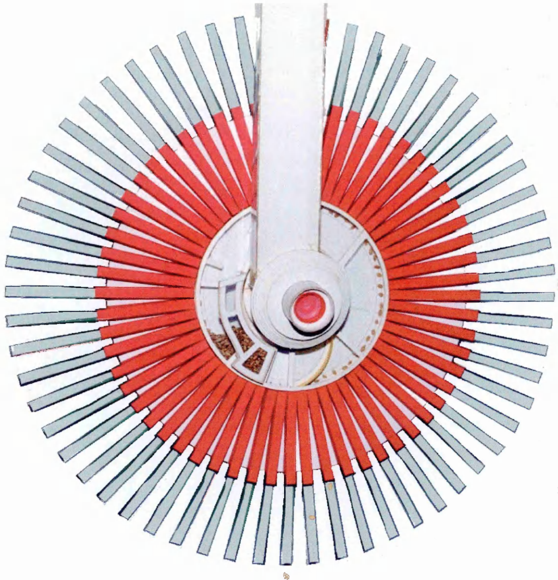
Plate 4.1. Working model of the delivery punch wheel with seed metering unit
