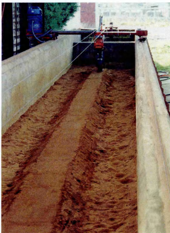
Plate 5.2. Precision punch planter prototype ready to test
