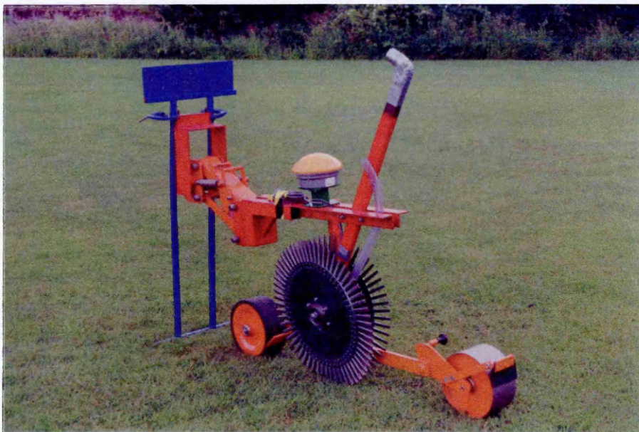
Plate 4.4: Precision punch planter prototype
