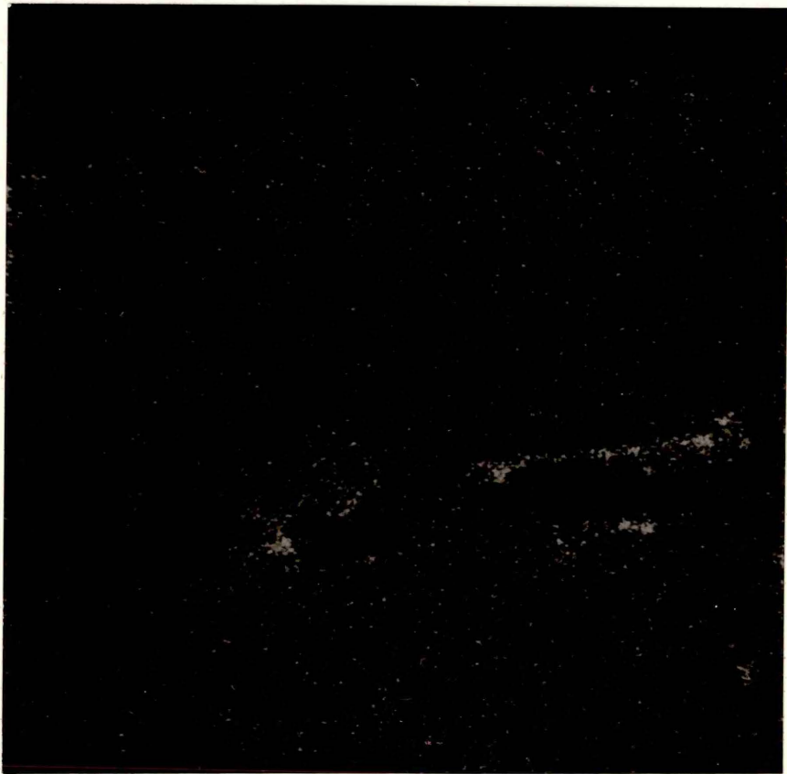
Fig. 4.10. Sulphur distribution in EN2 steel treated with sodium sulphate at 800°C
