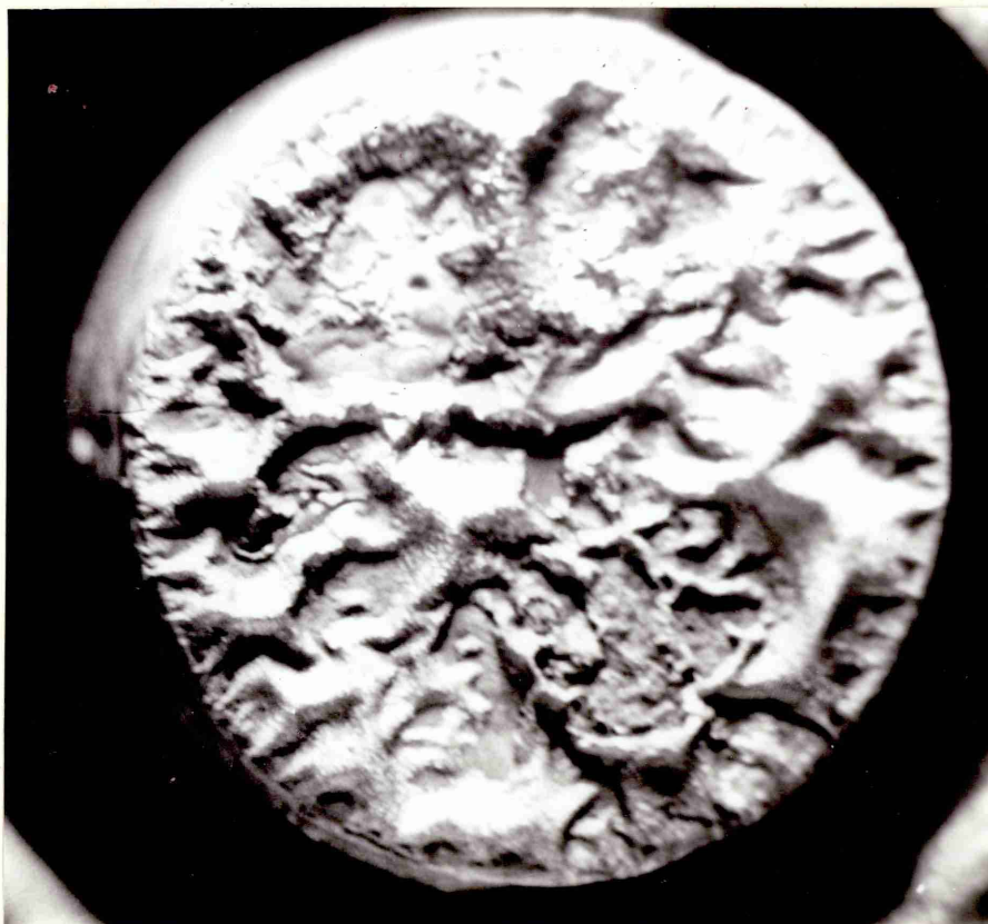
Fig. 4.8. Hot stage photograph at room temperature after sodium sulphate corrosion at 900^{\circ}\text{C} (Mag. x 11)
