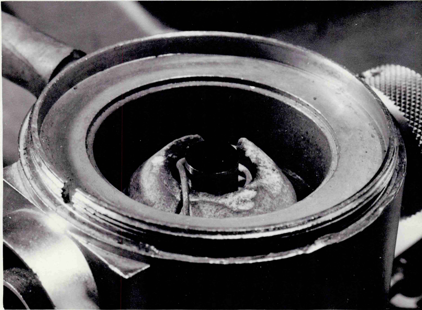
Fig. 4.1. Leitz hot stage showing specimen in position
