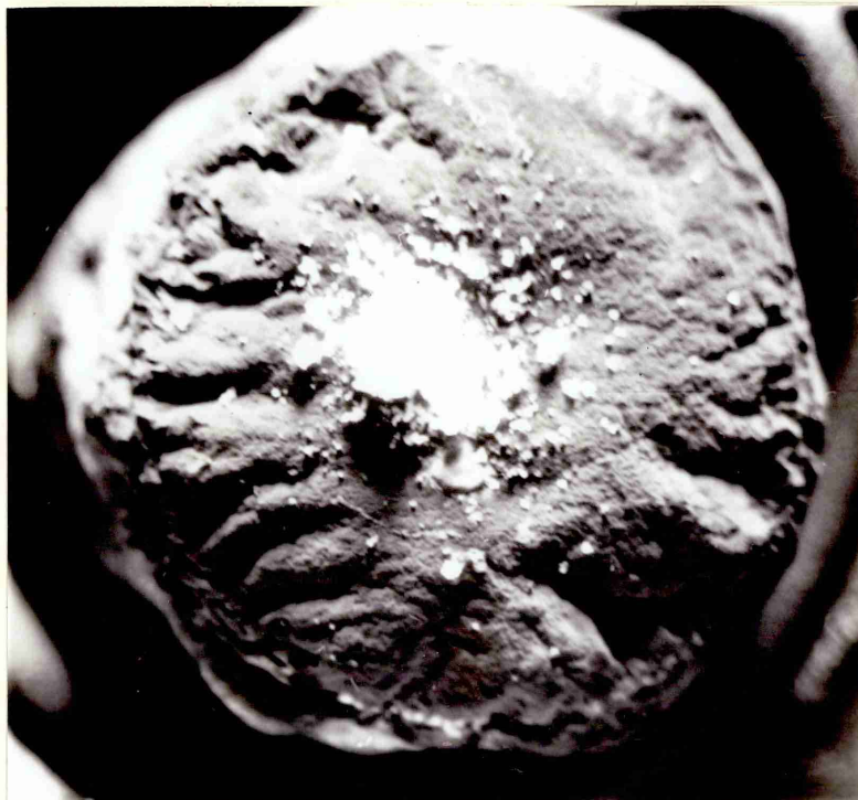
Fig. 4.8. Hot stage photograph at room temperature after sodium sulphate corrosion at 900^{\circ}\text{C} (Mag. x 11)
