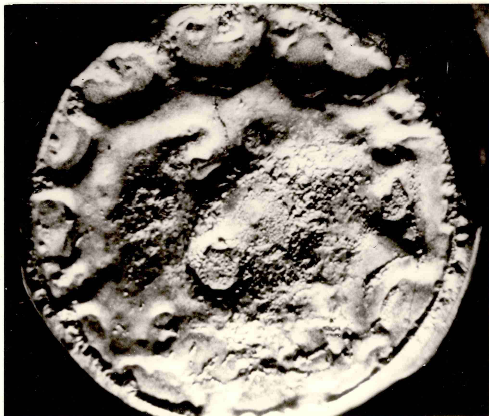
Fig. 4.3. NaCl on polished EN2, at 600°C during heating to 900°C (Mag. x 12)
