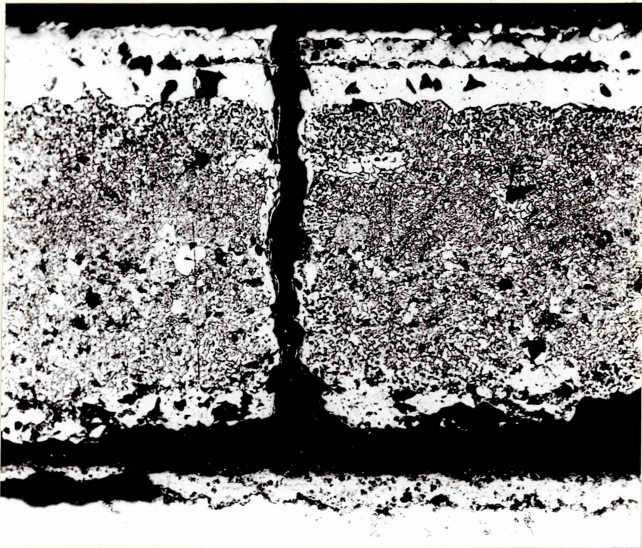
Fig. 3.21. Micrographs of cracks produced in oxide on EN2 steel by tensile loading (Mag. x 200)
