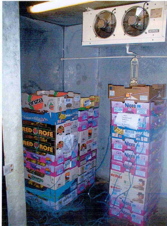
Figure 2.3 Fruit boxes stacked randomly in a constant temperature room. The wires leading into the boxes are thermocouple wires for temperature measurement.
