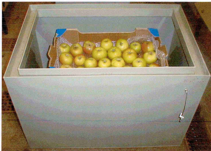
Figure 2.1 'Bramley' apple fruit in cardboard fruit trays inside a rigid polypropylene fumigation chamber. The tube and tap allowing samples of chamber atmosphere to be removed for 1-MCP quantification by gas chromatography (GC) can be seen on the front wall of the chamber. The trough around the top of the chamber was \frac{3}{4} filled with water and the lid (not shown) fitted into this, submerged under the water, forming the seal. A small fan was attached to the underside of the lid to facilitate air circulation within the chamber. Each chamber could accommodate 4 trays, each of which contained 30 fruit, giving a total treatment of 120 apples per chamber.
