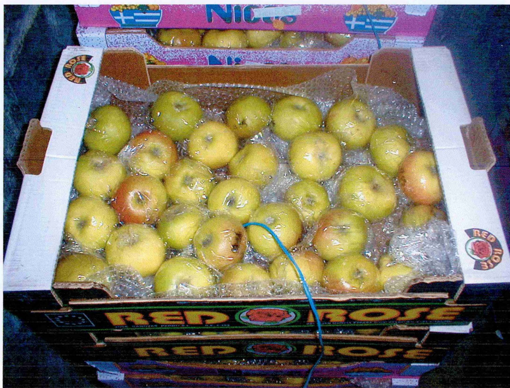
Figure 2.2 ‘Bramley’ apple fruit wrapped in perforated polypropylene bags, ready for storage. The wire leading into the box is a thermocouple wire for temperature measurement. Black markings visible on some fruit are identification numbers.
