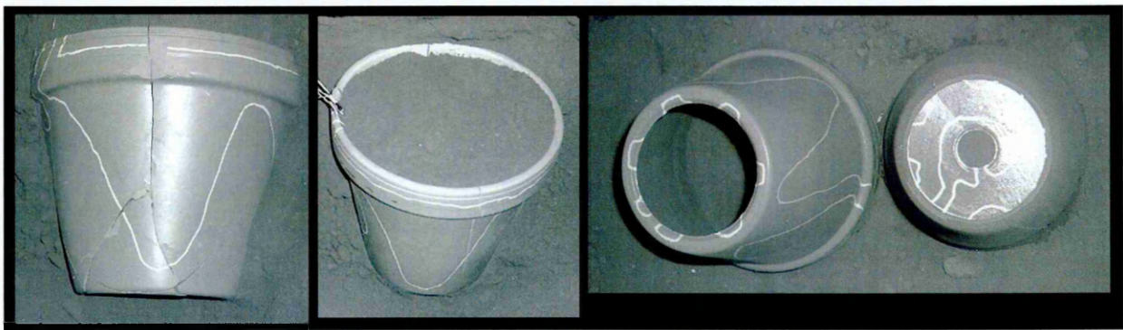
Figure E.5: Examples of broken pots and fracture patterns: Left to right: Horizontal, 45°, Vertical.
