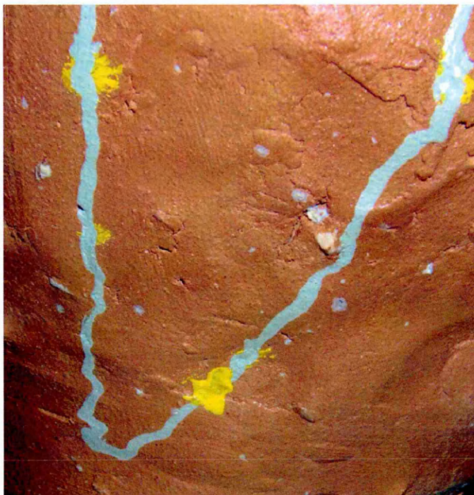
Figure 3.5: Application of yellow viscous paint with the conductive paint.
