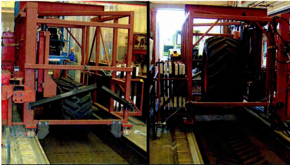
Figure 1.4. Soil bin laboratory showing both a rubber track (left) and combine harvester front tyre (right). (Ansorge and Godwin 2008).
