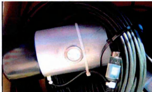
Figure 3.2: Pressure sensor mounted in the aluminium cylinder.
