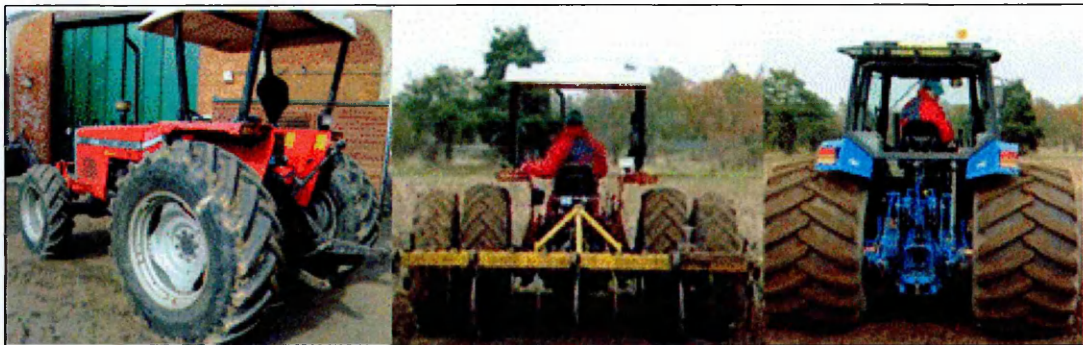
Figure 1.10. Single, dual and terra tyres used in the clay field experiment.
