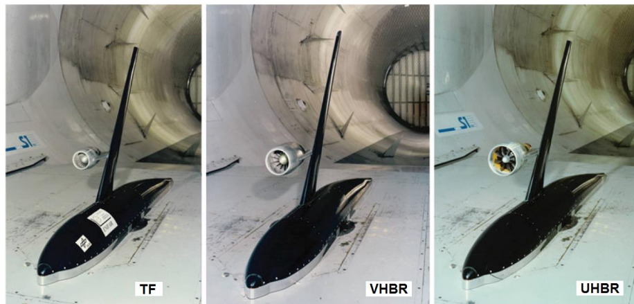
Figure 2-48: View of the three engine simulators mounted to the DLR-ALVAST airframe [75]
