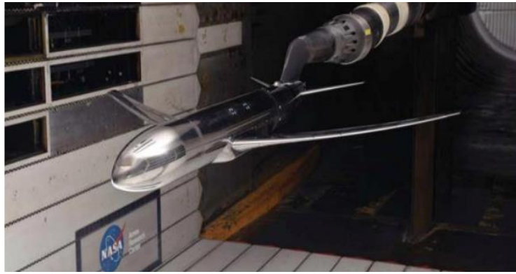
Figure 2-50: Clean-wing CRM in NASA's Ames Research Center Unitary Plan Wind-tunnel [82]
