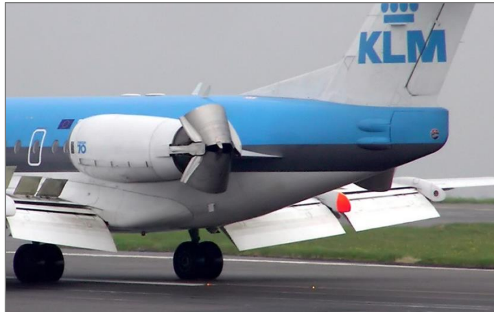
Figure 2-20: Bucket reversers deployed on a Fokker 70 [33]
