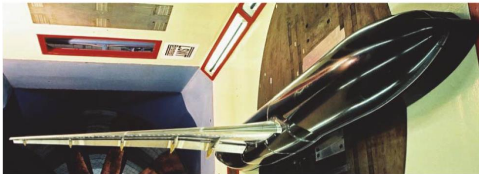
Figure 2-51: DLR F11 in the Airbus-Deutschland low-speed wind tunnel (B-LSWT) [84]
