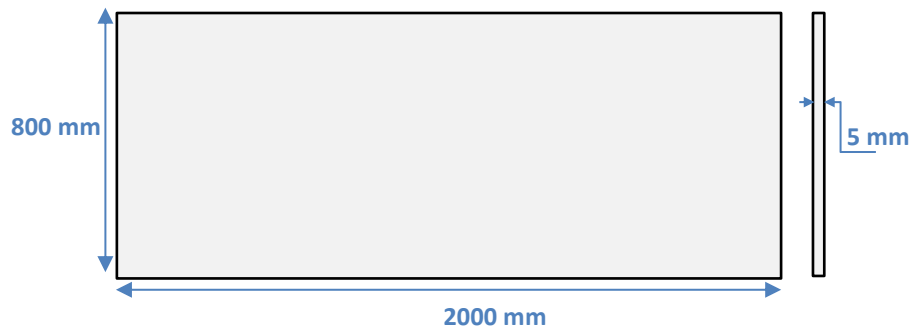
Figure 3-38: Dimensions of the spoiler plates
