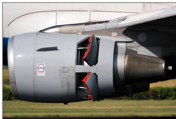
Figure 2-18: CFM-56-5 turbofan with deployed reversers [32]
