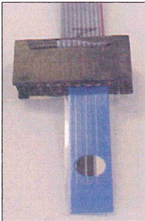
Figure 2.3 Standard electrode connector allowing electrode linkage to the electrochemical analyser
