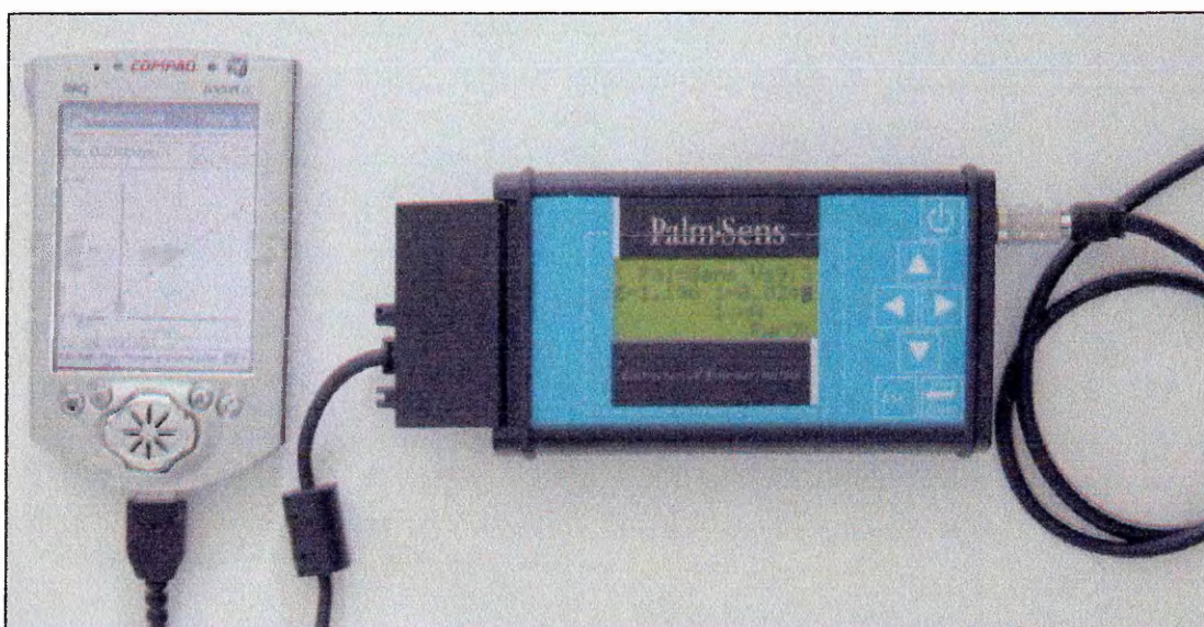
Figure 4.2 PalmSens electrochemical analyser (dimensions: 155 mm x 85 mm x 35 mm; weight: 0.45 kg; power: 2 AA cells NiMH for 6-8 hrs operation).
