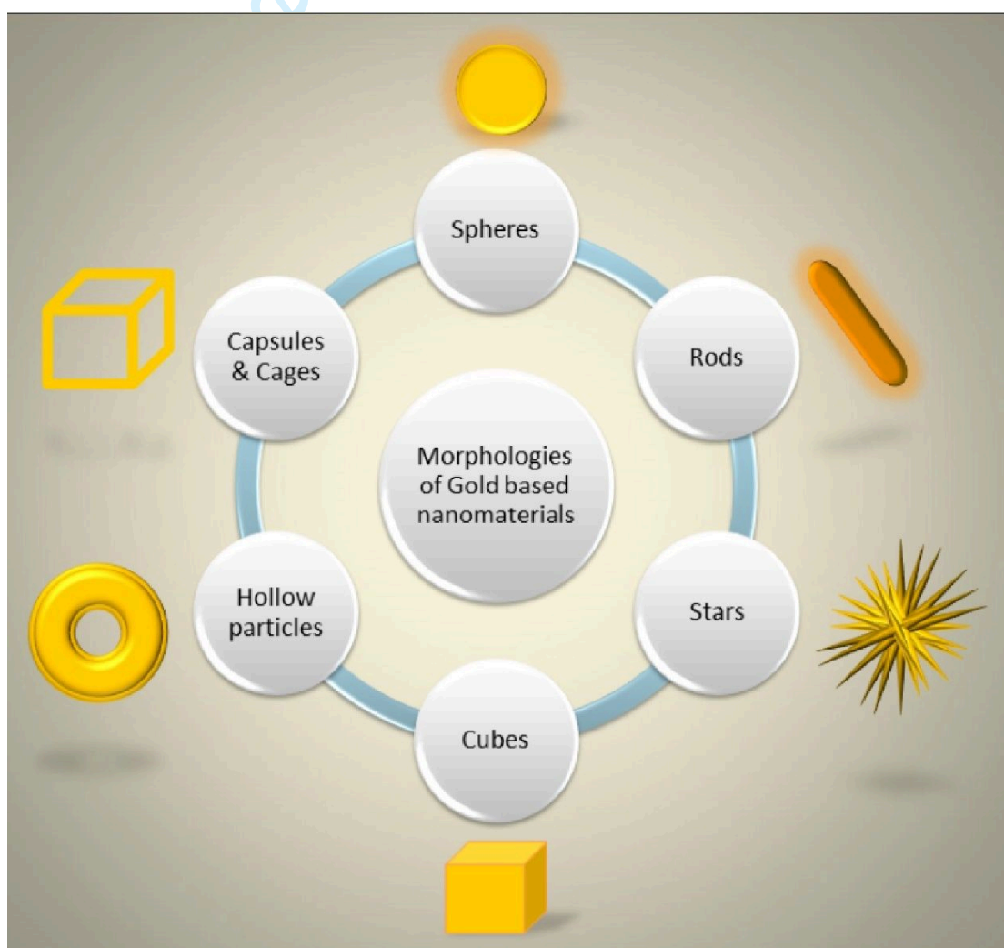
Figure 6 Schematic representation of the main morphologies of gold-based nanomaterials [84]:
