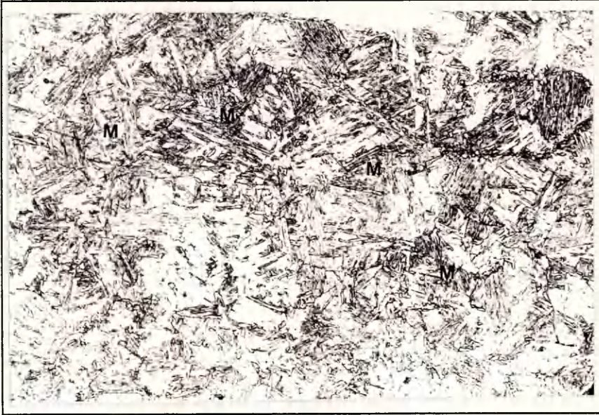
Fig. 8.8(a) Steel 12 HI= 0.8kJ/mm Hv= 371-336 359.6 300X
