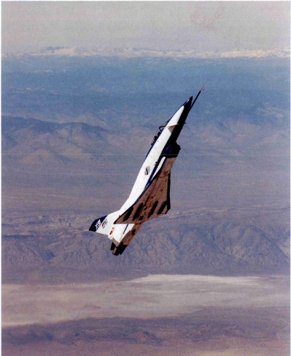
Dryden Flight Research Center EC94-42478-4 Photographed 1994 X-31: Demonstrating entry into the high angle of attack Herbst Maneuver. NASA photo by Jim Ross
