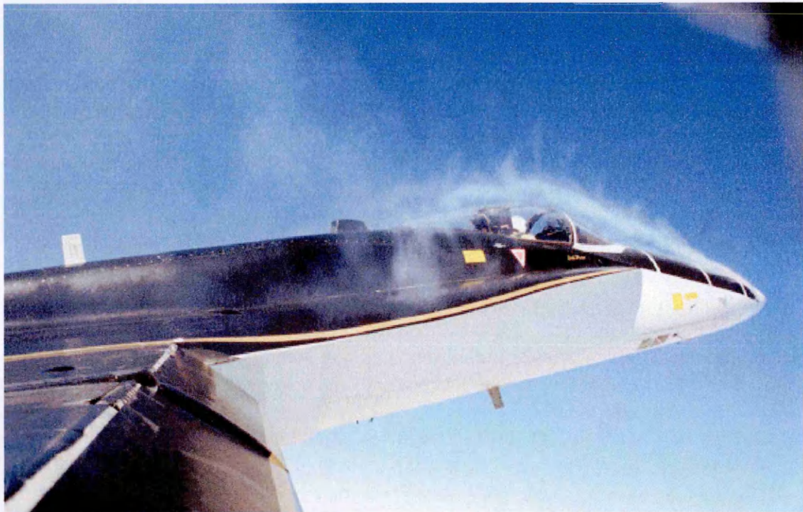
Figure 1: Forebody vortex flow visualisation using smoke on the NASA F-18 High Alpha Research Vehicle (HARV) at \alpha = 42^\circ . NASA photograph.
