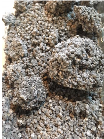
Figure 2-3 Photograph of cemented steel slag from the column with 1.75 mm sized media.
