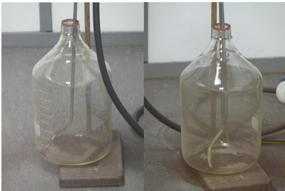
Figure 4-8: The Glass Durham bottle when the compost material was not close to the pipe (the right picture) and when the compost was close to the pipe (the left picture), and therefore the emissions concentration was affected by this factor.
