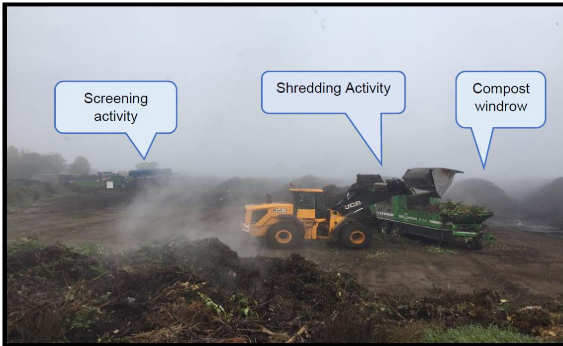
Figure 5-1: Ramsey Composting site during the shredding activity. The agitation activities during the sampling visits were turning and screening, turning only, and shredding and screening during the first, second and third sampling visit respectively.
