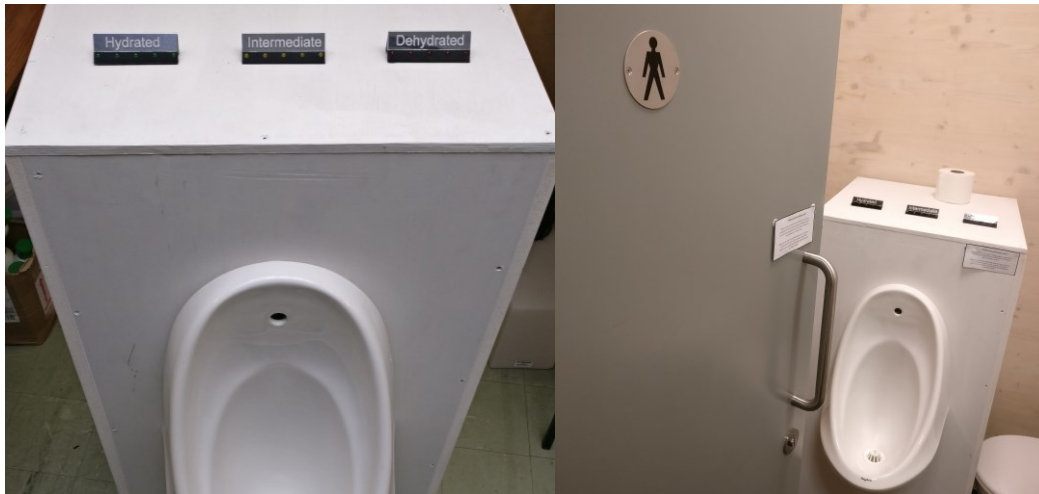
Figure 6-20 Experimental test prototype with traffic light signals.
