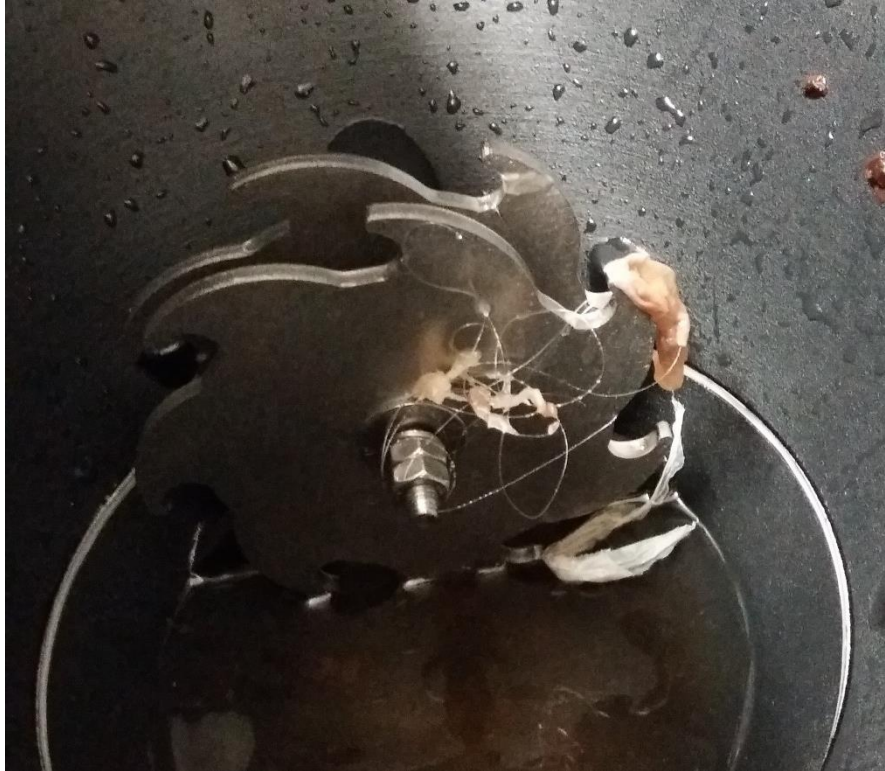
Figure 14. Macerator 7 th test Nylon thread entanglement
