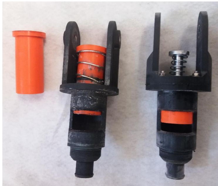
Figure 20. Original Plunger/ Feeder vs V2 Feeder
