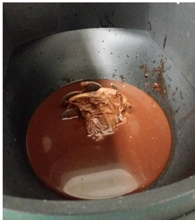
Figure 11. Macerator 3 rd test paper caught on exposed shaft
