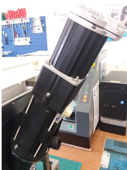
Figure 17. The motorised version of the screw with a flexible coupling
