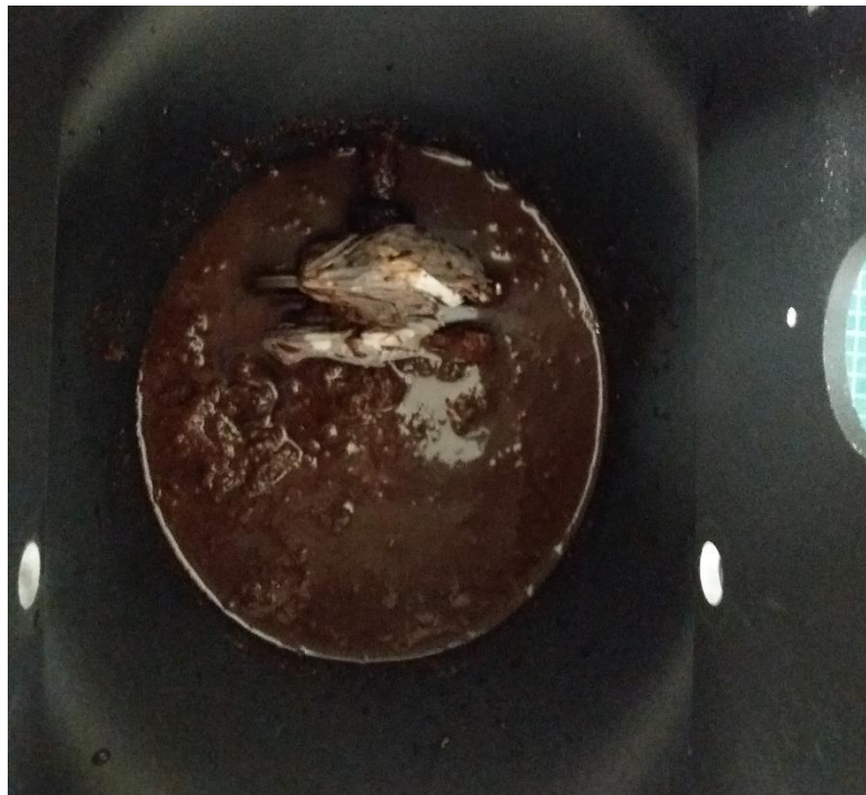
Figure 13. Macerator 6 th test plastic bag entanglement
