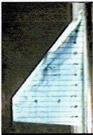
Delta 70, B.L.=14mm, k=0.05, AOA=20deg. UP
