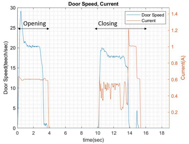
Figure 3: Door speed and current signals of the opening and closing operation.
