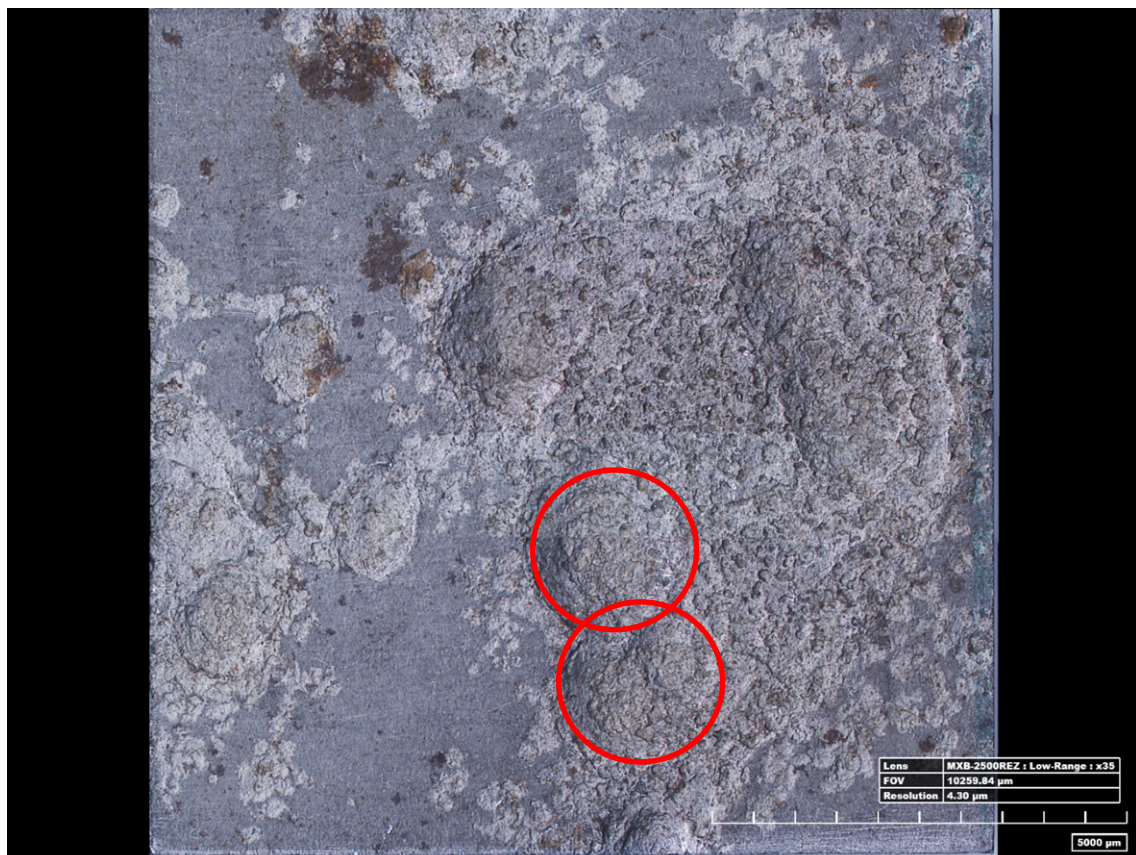
Figure 5-13: Pit coalescence represented by the red circles(each showing a pit) that are now joined to form a new pit.
