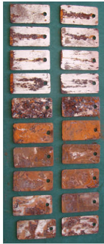
Figure 2-16: Rusted coupons from wind farms [127]
