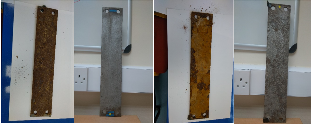
Figure 5-16: Difference between clean and dirty plates
