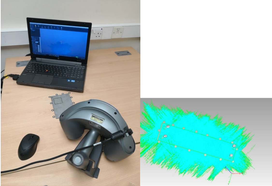
Figure 5-30a & b: Laser scanning tool and raw data cloud
