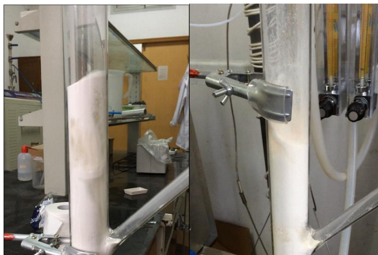
Fig. 3-3 Fluidization of silica sand particles (~0.2mm and ~0.3mm) at the carrier gas flowrate of 360L/h
