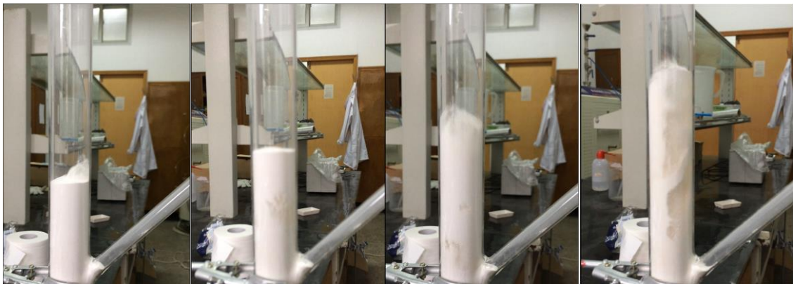
Fig. 3-4. Cold state tests of silica sand particle (~0.2mm) with different gas flowrates (selected presenting: 100L/h,200L/h,300L/h and 400L/h)
