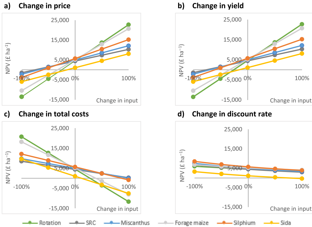
Fig. 2. Sensitivity of the NPV (over 16 years at 4% discount rate) of four bioenergy crops and an arable rotation including maize to changes in a) prices, b) yields, c) costs, and d) discount rates in the United Kingdom.
