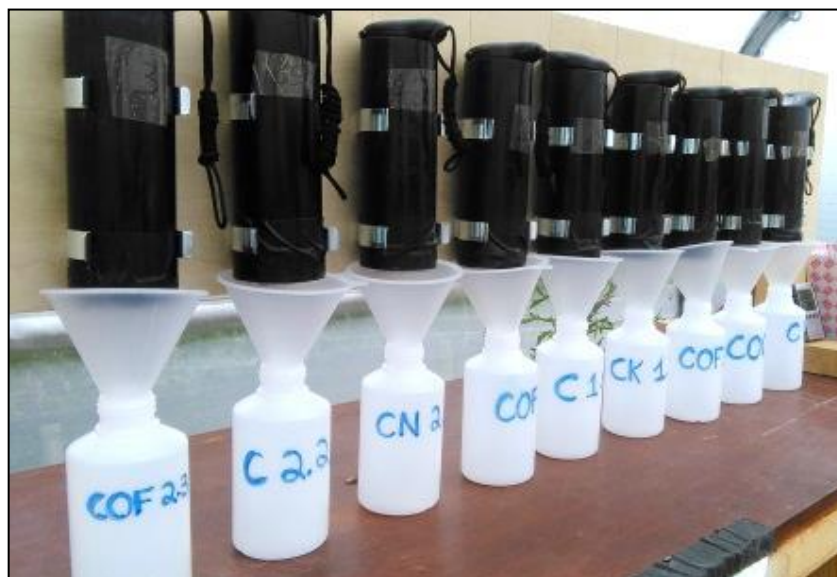
Figure 4.1. Column trial experimental set-up.
