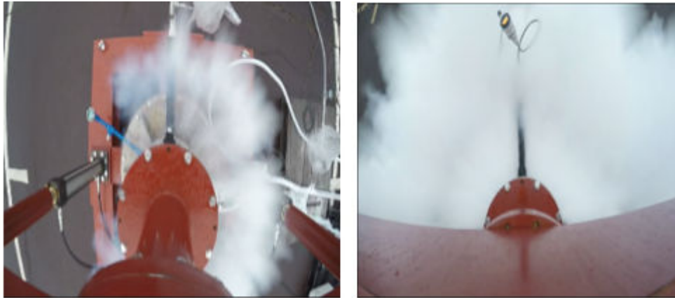
Fig. 10: Top view of the release of Test 1.1 (left) and Test 2.1 (right) after 0.01 s of the vessel separation
