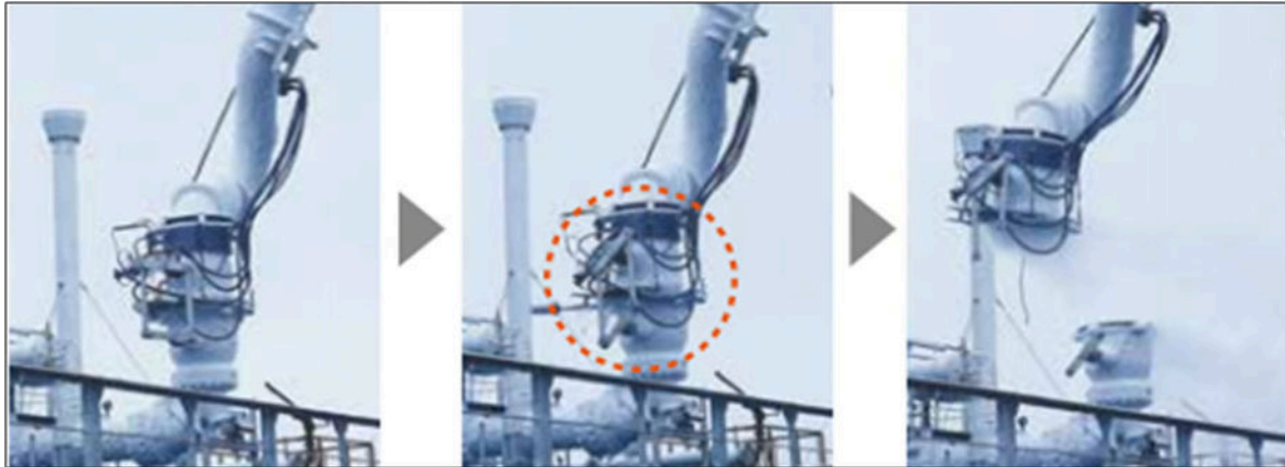
Fig. 3: Sequence of the operation of ERS; 1) separation begins; 2) the two valves shut completely; 3) Emergency Release Coupler opens completing the separation (Tokyo Boeki Engineering, n.d.).
