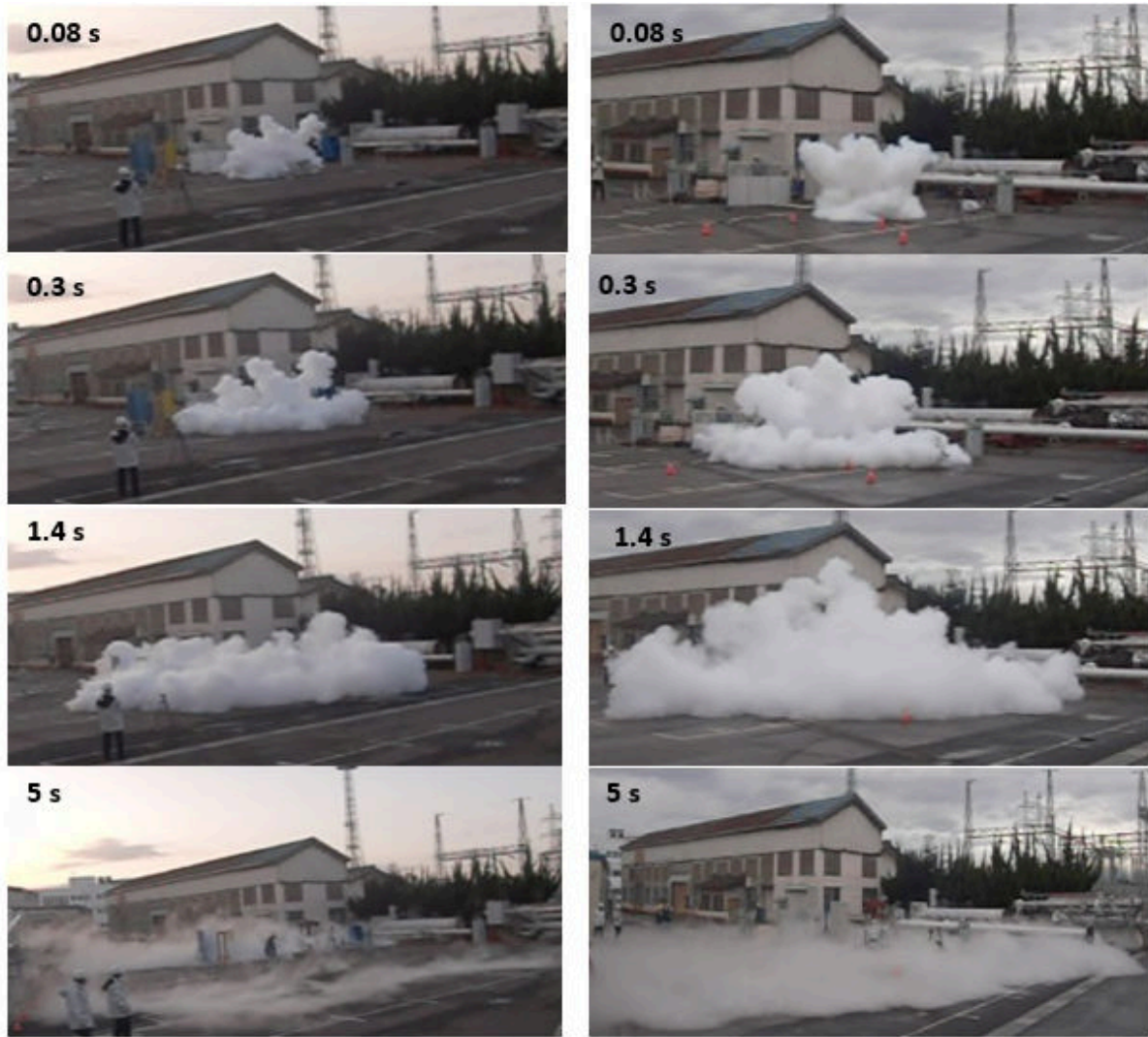
Fig. 21: Dispersion stage of the release in Test 1.2 (left) and Test 2.1 (right)
