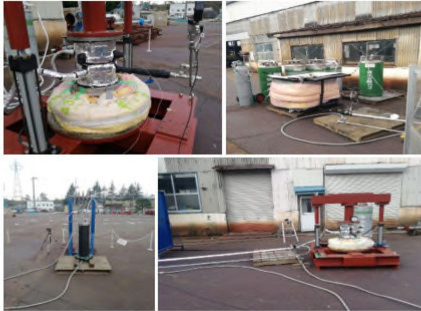
Fig. 5: Pictures of the experimental apparatus - left-to-right and top-to-bottom: test vessel; methanol-nitrogen refrigeration; buffer container; inlet, outlet pipework and pressurised oil system
