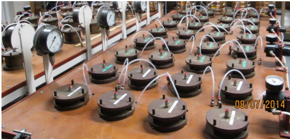
Figure 6 Photo of pressure cells used for determining water retention characteristics.
