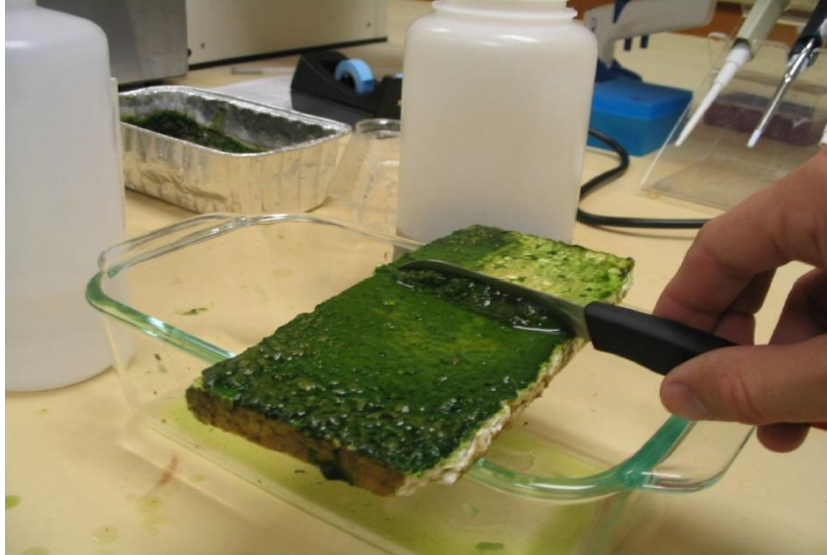
Figure 13 Removing microalgae biofilm from attached cultivation system [181]
