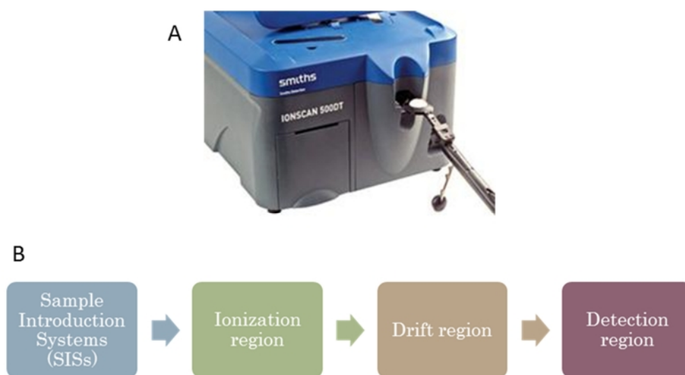
Figure 1-8: (A) Commercially available IMS (IONSCAN500DT - Smiths Group plc., UK) and (B) illustration of the principal IMS components.
