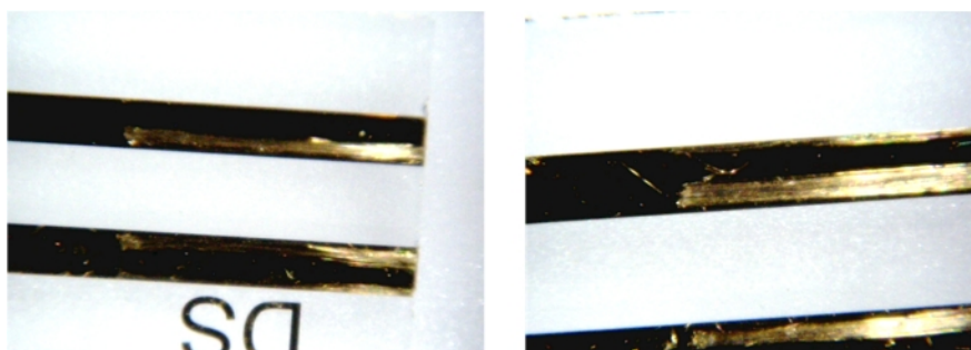
Figure 2-9: Image of the DPR IDEAu5 electrodes, showing the damages of the connections.
