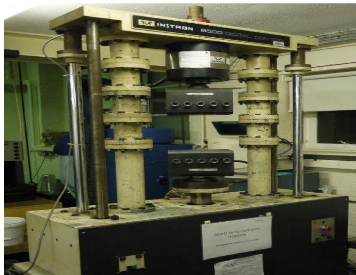
Figure 3. 21 250 KN INSTRON 8500 test rig (Boeing standard 4ASTM D 7137).
