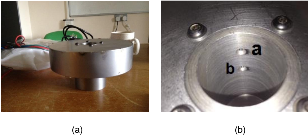
Figure 3. 11 Optoelectronic device: (a) overview; (b) two holes containing light-producing diode (LED).
