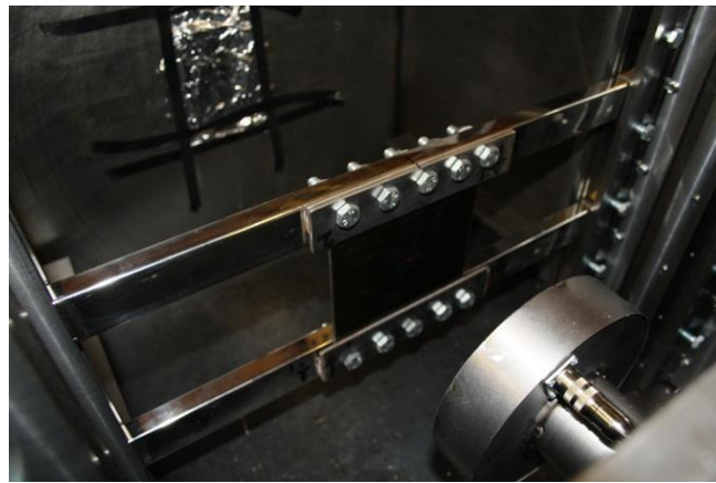
Figure 3. 15 Adjusting the centre of composite laminate in the path of projectile.
