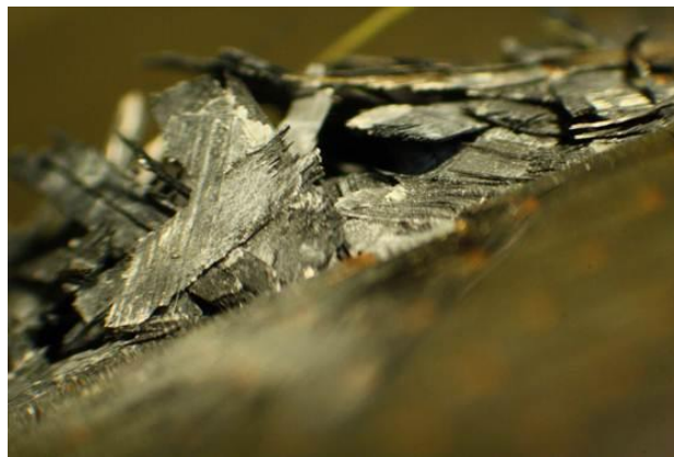
Figure 3. 20 Micrograph of impact failure of 7 layered CFRP woven compost laminate impacted at 141 J (200 m/s).
