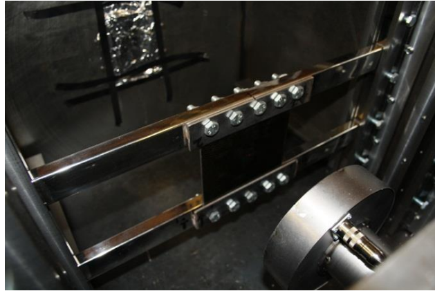
Figure 3. 13 Support frame with composite laminate in gun system.
