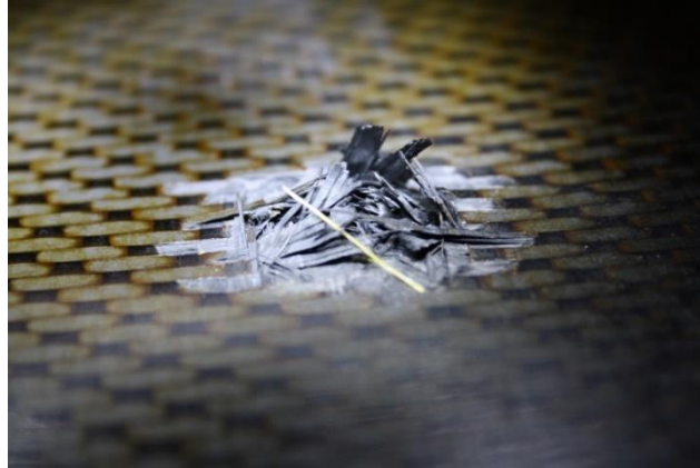
Figure 3. 19 Petalling formation failure of 11 layered CFRP woven compost laminate impacted at 141 J (200 m/s).
