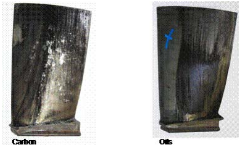
Figure 2-3: Different types of fouled compressor blades [13]
