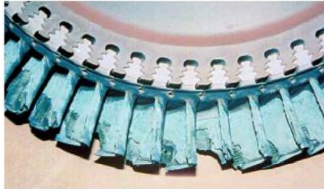
Figure 2-6: Hot Corrosion on a Turbine Rotor [28, p.175]
