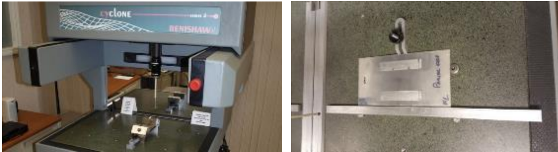
Figure 3.11 Surface mapping scanner and the clamping system of a DSR sample
