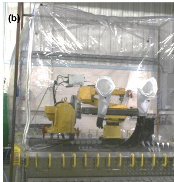
Figure 2-27: WAAM set – up (a) in open air; (b) in an enclosure
