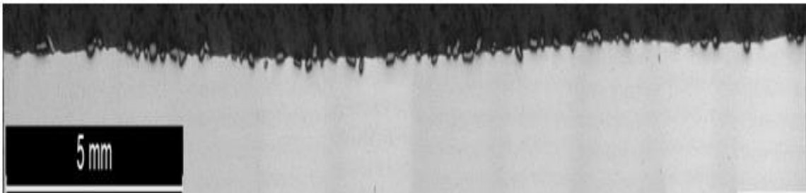
Figure 6-16: Longitudinal micro section of the top surface of melt bead showing 150 \mu m SiC particles at the top of weld bead (WFS: 2.8 m/min)
