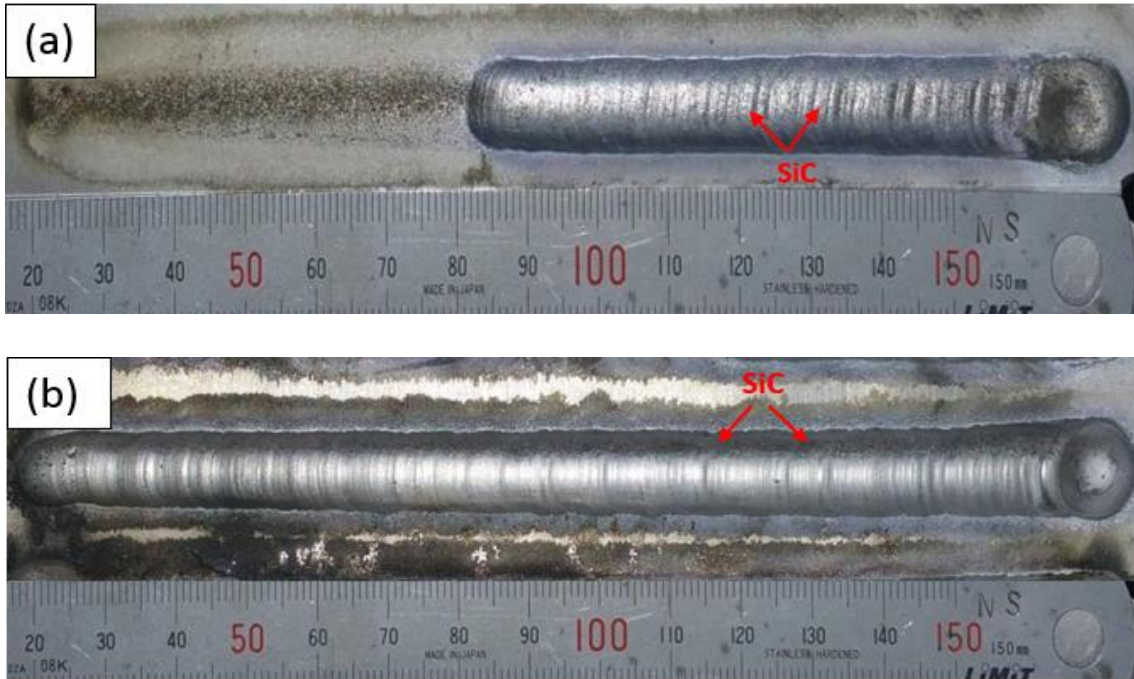
Figure 6-3: Melt seam tracks produced by injecting particles at different positions (a) back and (b) side of melt pool
