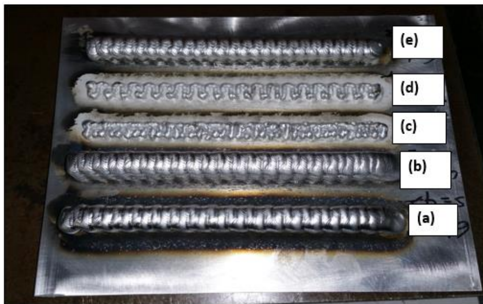
Figure 4-15: Physical features of walls built by oscillating in CMT-PA mode: (a) WFS/TS=10; (b) WFS/TS=15, (c, d) WFS/TS= 5 and (e) WFS/TS=20
