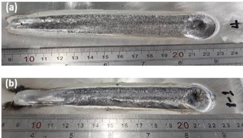
Figure 6-13: Physical characteristics of Al-SiC composite weld seam tracks produced using 150 μm SiC (HI = 1.6 kJ/mm; V_{SiC} = 2.9 m/s; PFR = 22 g/min): (a) autogenous weld seam (b) Filler wire (WFS = 2.8 m/min)
