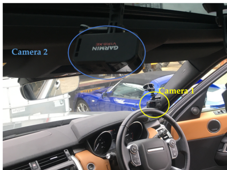
Figure 5. A illustration of the two cameras inside the vehicle.
