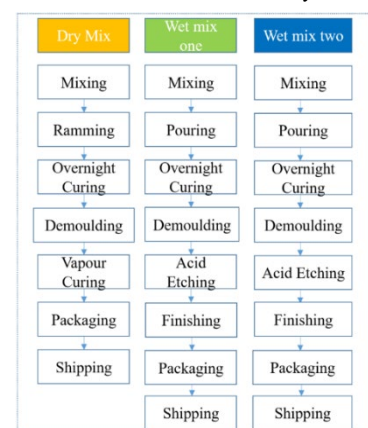
Fig. 3. Cast stone manufacturing process
