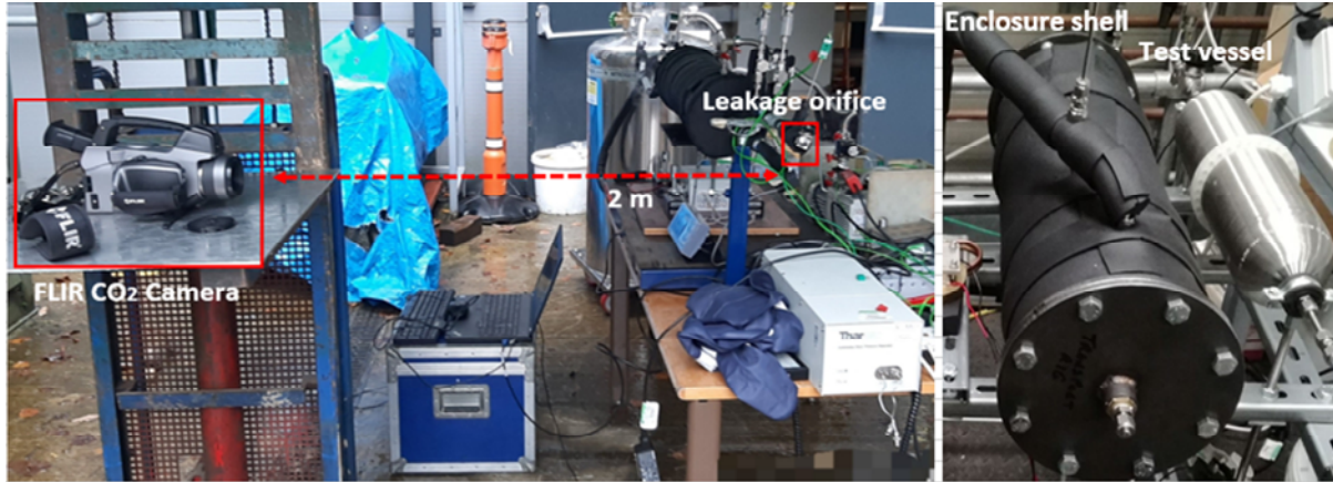
Figure 3: left-to-right CO 2 camera acquisition view; enclosure shell and test vessel prior to assembly
