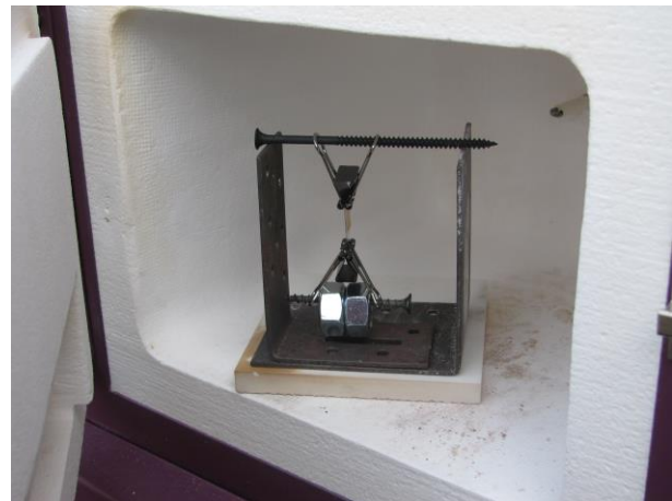
Fig. 15: Thermomechanical Demise Test Set-Up
