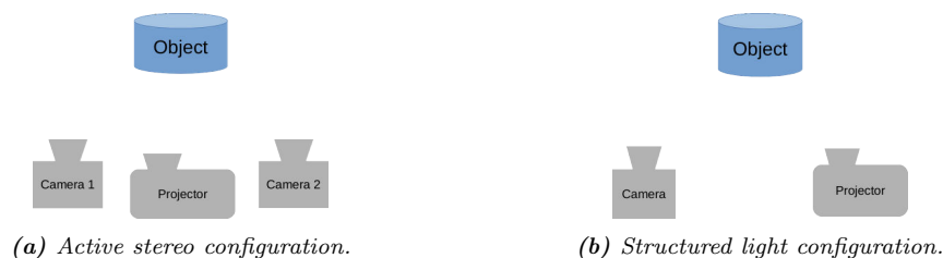
Figure 7: Common active triangulation configurations.
