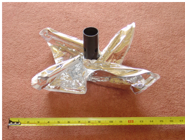
Figure 3-15 Phased deployment of a small rib-wrap demonstrator
