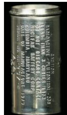
Figure 8-2 A Plutonium-238 RTG for use in a cardiac pacemaker
