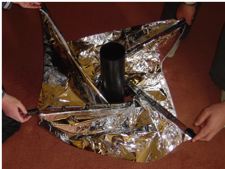
Figure 3-13 The possibility of loose fabric fouling the motion of a large rib-wrap pattern deployment demonstrator is apparent in this photograph
