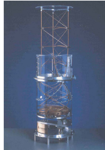
Figure 3-23 Coilable Mast system, reproduced from Tilbert (2002)
