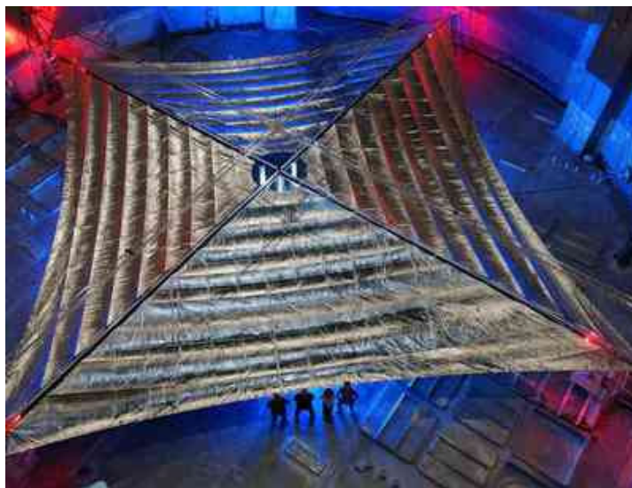
Figure 3-9 The 20 m L'Garde solar sail demonstrator (picture credit NASA MSFC)
