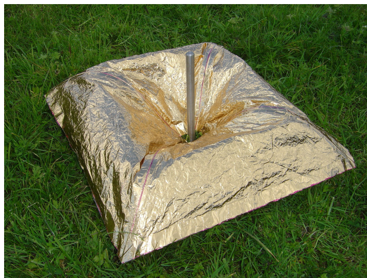
Figure 3-10 Tension in the membrane edges stalling the deployment of a small Miura-Ori pattern deployment demonstrator. This semi-deployed shape remains stable even if the demonstrator is inverted.
