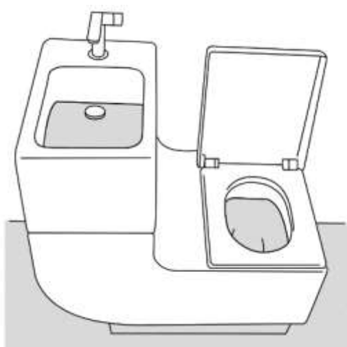
Figure 13 - Example of hand washing reusing sink to reduce grey-water (Tierney, R. 2017)
