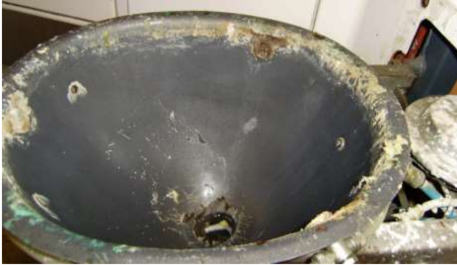
Figure 101 - Calcite deposit in train toilet after three years and at least 28,000 uses.
