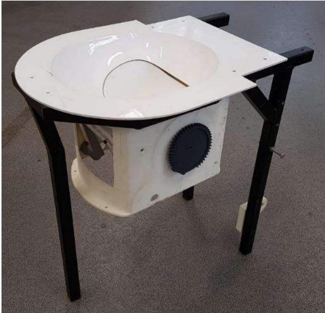
Figure 43 – Photo of user interface of P2 for testing swipe performance with metal support frame. (Tierney, R. 2017)
