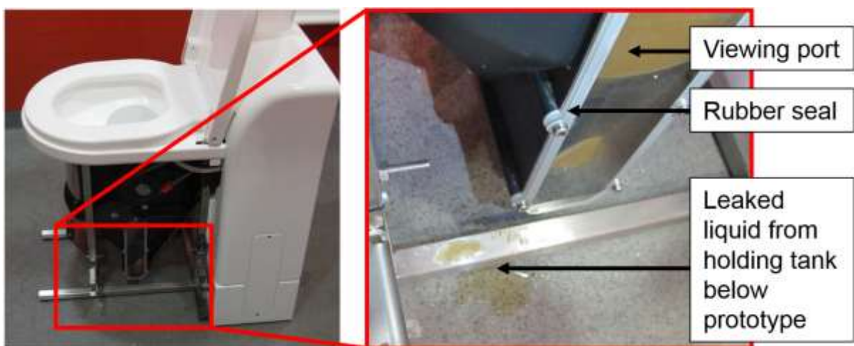
Figure 72 - Photograph of toilet prototype and enlarged area under prototype where liquid leaked from the holding tank overnight due to loose seal on the viewing port. (Tierney, R. 2017)
