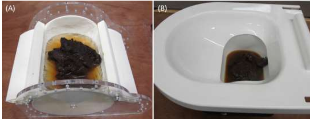
Figure 44 – Testing both prototypes (A) P1 (B) P2 with 500g of soybean paste and 200ml of water to simulate urine. (Tierney, R. 2017)
