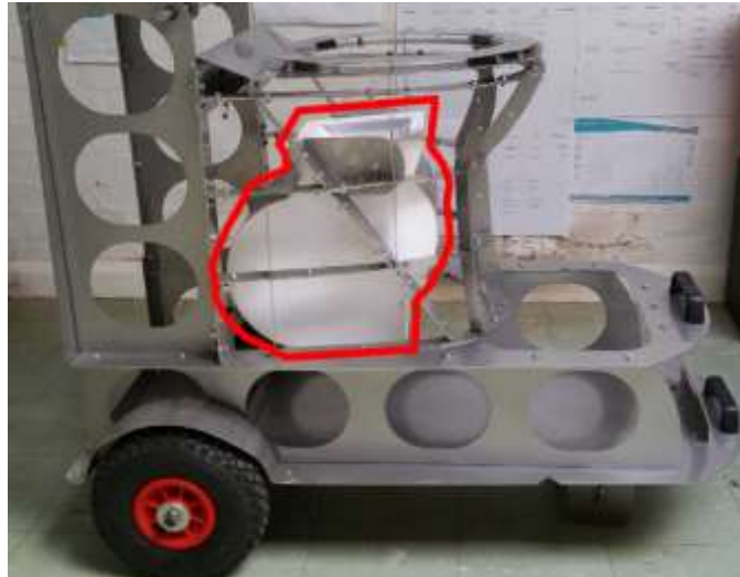
Figure 35 – Integration testing with cardboard modular prototype inside aluminium skeletal toilet frame with red outline for clarity. (Tierney, R. 2017)
