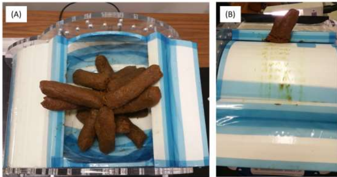
Figure 39– (A) 750g of soybean paste in the bowl of P1 (B) 750g of soybean paste at the point of failing the MaP test
