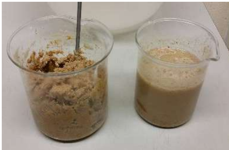
Figure 94 - Simulant faeces samples following the sponsor recommended recipe. Sample on the left is 60% solid. Sample on the right is 25% solid.
