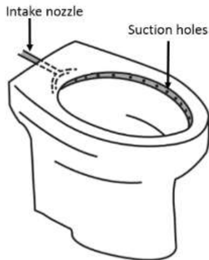
Figure 16 - Odour extraction testing (Seo & Park, 2013) (Tierney, R. 2017)
