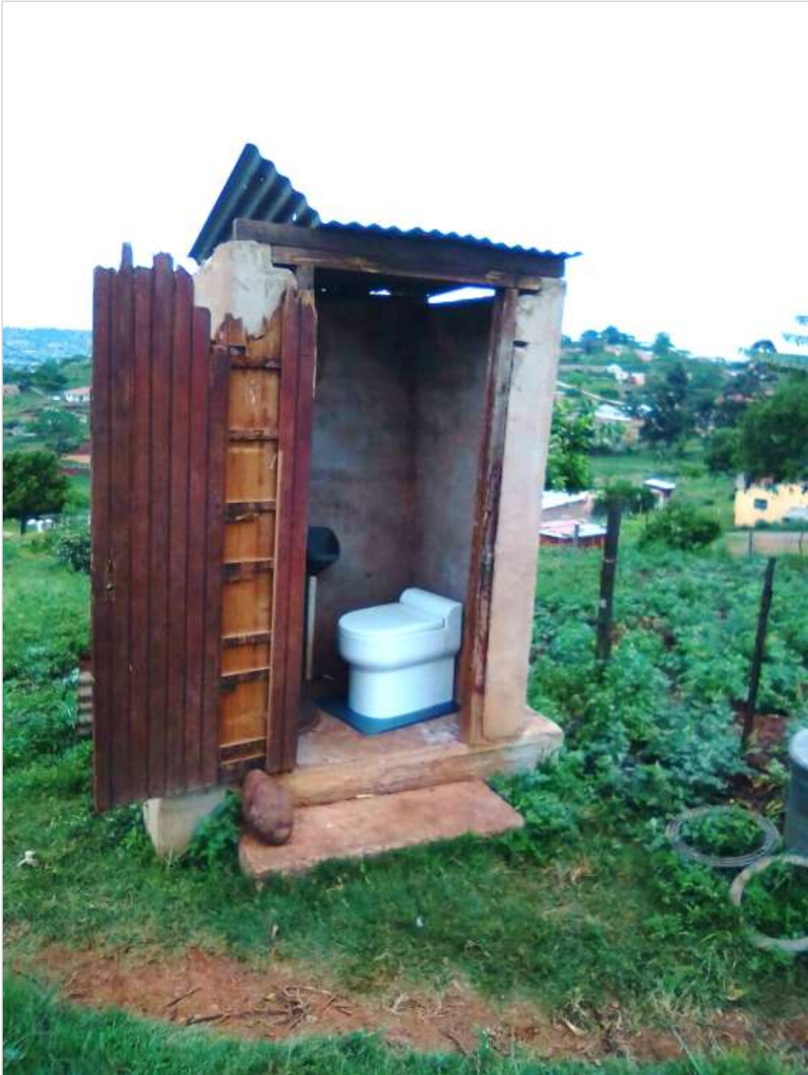
Figure 93 - The Nano Membrane Toilet user interface in an undisclosed location in Africa ready for the next set of user testing as the project continues. (Image courtesy of Jan Henning, 2017)
