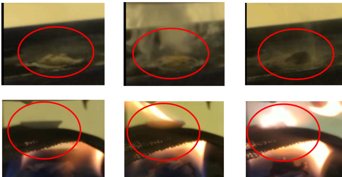
Figure 5-9 The top row shows different stages of the burning of Formulation 1 without an accelerant: melting at 25 s (left), massive gaseous production from decomposition and burning at 1 min 47 s (centre) and residues (right); the bottom row shows three stages of burning on top of a sieve saddle: early/12 s (left), middle/19 s (centre) and full burning/30 s (right)
