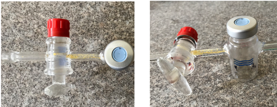
Figure 5-8 Example of DNAN condensed within the modified headspace vial
