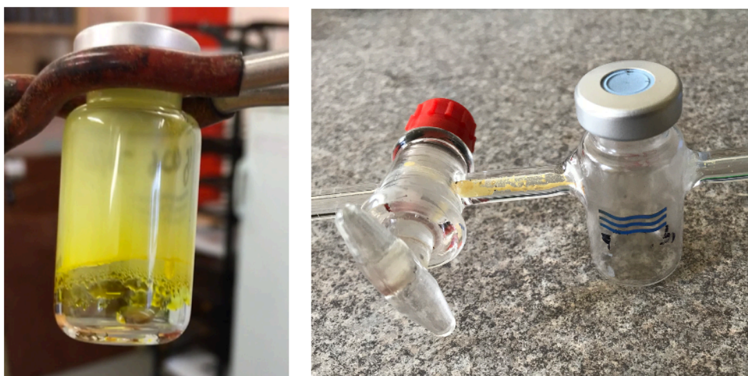
Figure 7-1 Recovered DNAN in the closed-system experiment (left) and open-system experiment (right)
