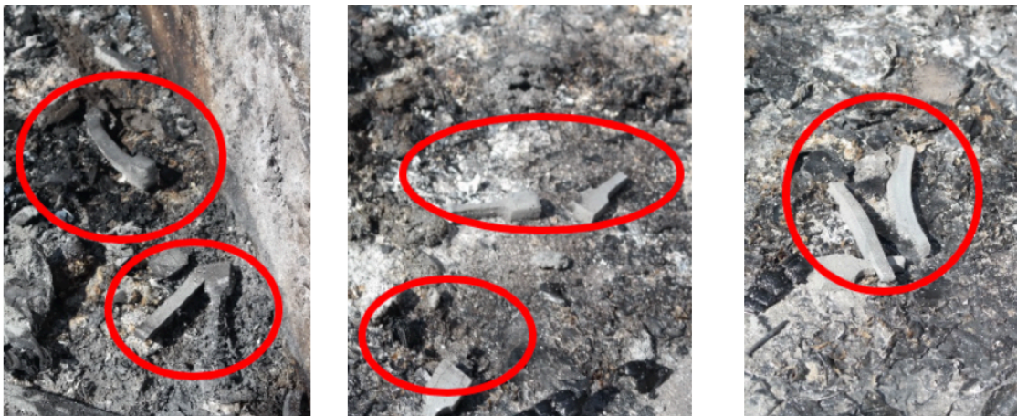
Figure 5-15 Photographs of the waste after burning with the remaining 'dog bone' samples of explosive: explosive residues after the first burning (left – day 4), second burning (centre – day 5) and third burning (right – day 6) – no explosive was added after the first burning (day 4)
