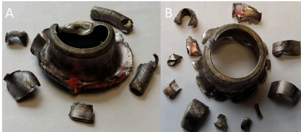
Figure 10. Recovered neck and fragments from 4-mm thick cylinders: A) mild and B) stainless steel.
