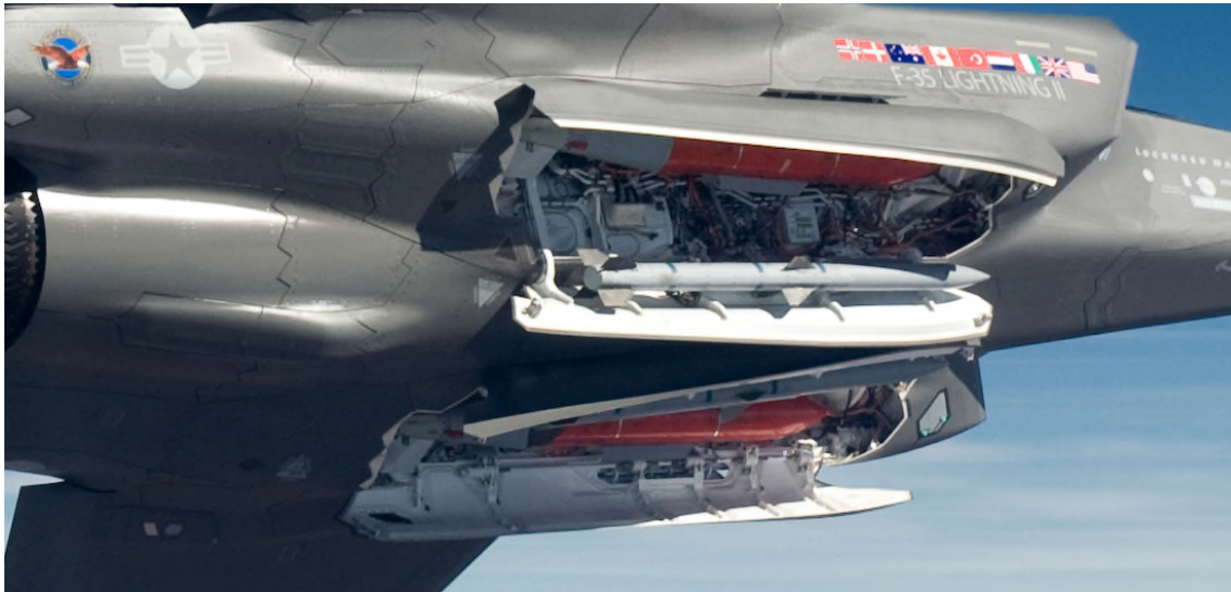
Figure 2.17 – Close-Up view of the F-35 weapon bay. (Image source: Google Images®)
