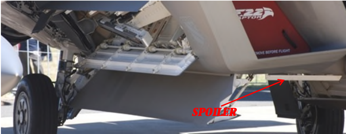
Figure 2.15 - View of the F-22 main weapon bay with spoiler extended. (Image source: Google Images®)
